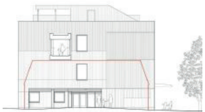
Above: West elevation. The outline of the existing building is indicated in red.
